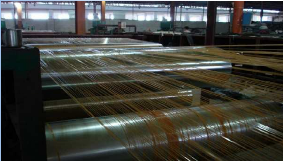
The film is then spun into 5mm thick thread
