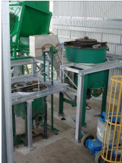
Magnet Conveyor & Caustic Wash Tank
