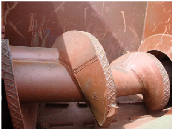
Primary Auger of Komar Shredder
