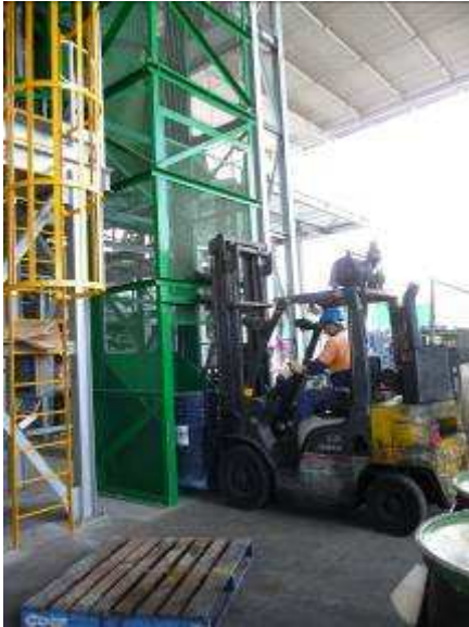
Loading Drums into Skip lift with Forklift
