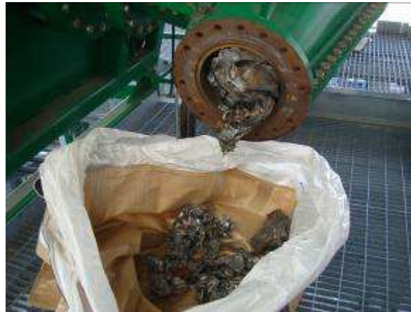
Shredded Metal Exiting Secondary Auger
